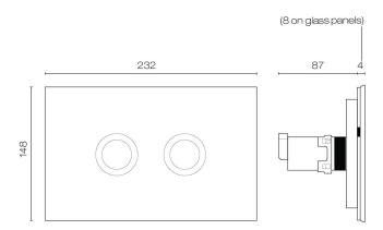
Note - Minimum wall thickness of 20mm
